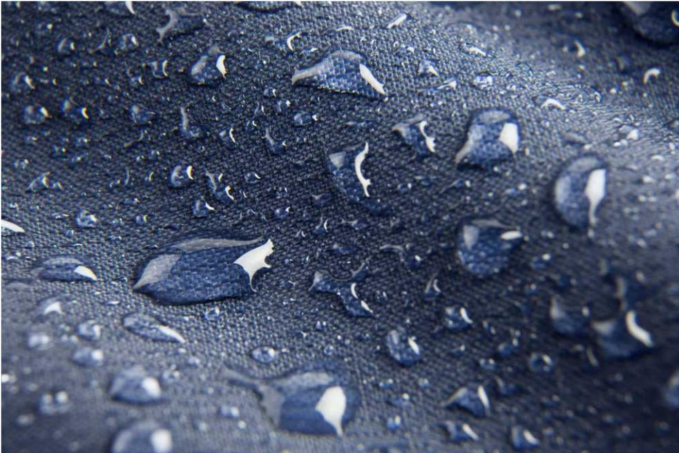
Modifying the way textiles interact with water is a fundamental product differentiator. This report discusses super-hydrophobic surfaces used to create self-cleaning materials, faster-drying textiles, and improved stain resistance.
